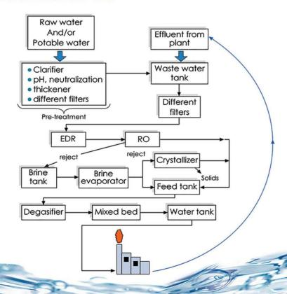
After the above mentioned treatments, using up to date and highly efficient processes, the several waters are fed to the water recovery unit, which consists of:
